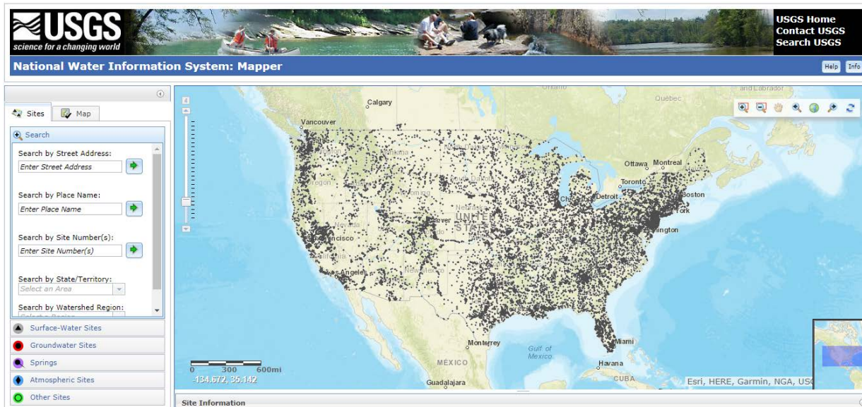
Figure A.3 Splash page for USGS's National Water Information System. The page allows users to select various USGS monitoring sites across the United States and access data such as streamflow, discharge, and field measurements at selected locations. SOURCE: https://maps.waterdata.usgs.gov/mapper/index.html , accessed September 6, 2018.
