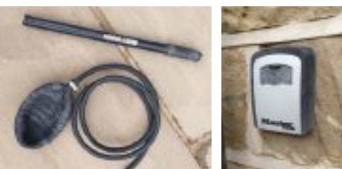
Toilet bung for use in the ground floor toilet and a key safe so neighbours can install barriers if owner is away.
