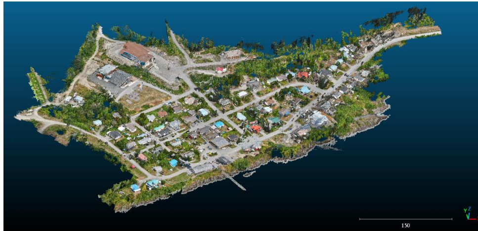
Figure 2: Overview of photogrammetry-derived point cloud for the Village of Gitwinksihlkw.
